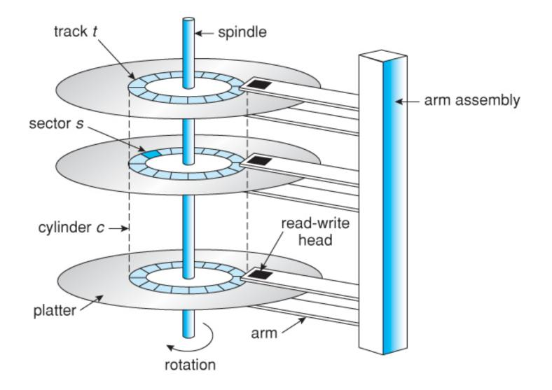
Cylinders: all the tracks under the head at a given point on all surface Head
