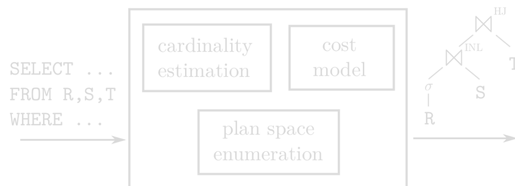
Figure 1: Traditional query optimizer architecture
